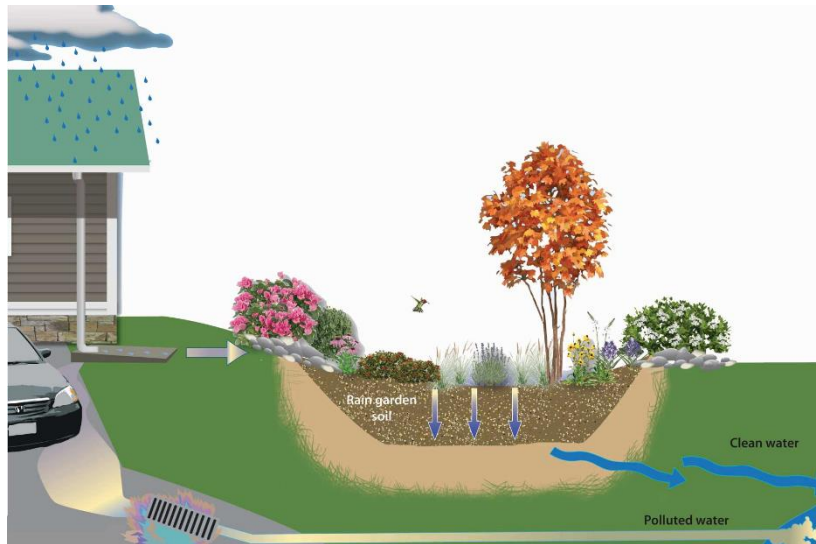
Figure 1 How a rain garden works
